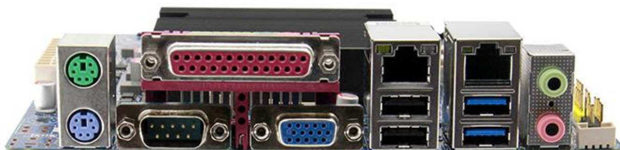
PS/2 COM1 PRINTER VGA LAN-USB1 LAN-USB2 AUDIO-JACK
